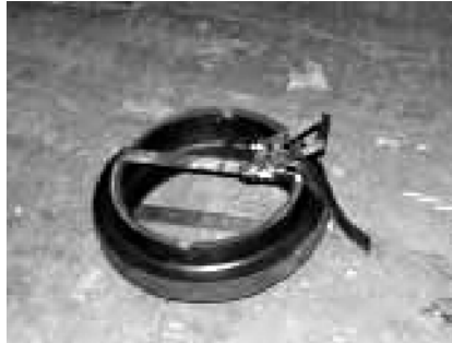
Figure 30. Feeding Strap End Through Slot in Hub Barrel
