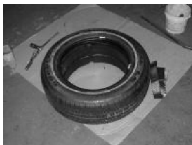
Figure 17. Preparing to Remove Runflat
