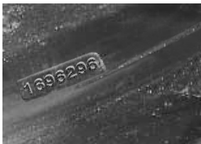
Figure 28. Runflat Serial Number Location
