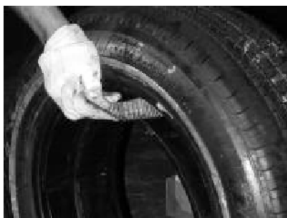
Figure 18. Pulling Strap Over Top of Runflat
