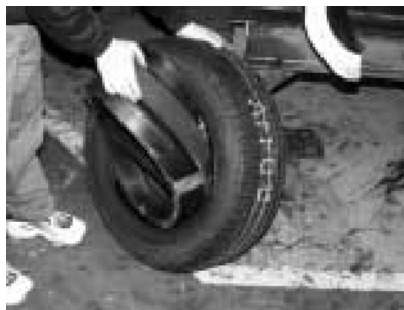
Figure 32. Inserting the Runflat into Tire Cavity
