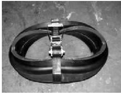
Figure 31. Compressing the Runflat
