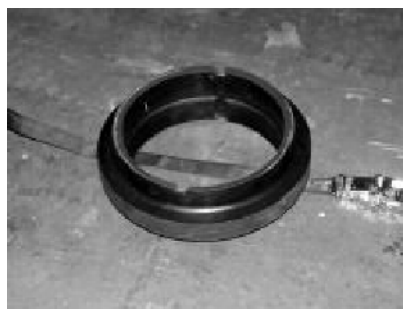
Figure 29. Preparing to Compress Runflat
