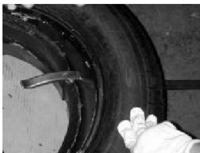
Figure 23. Resting Tire Iron Handle on Hard Surface
