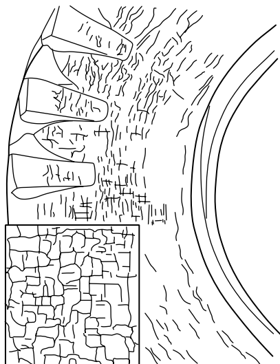
Figure 8. Oxidation of Sidewall
