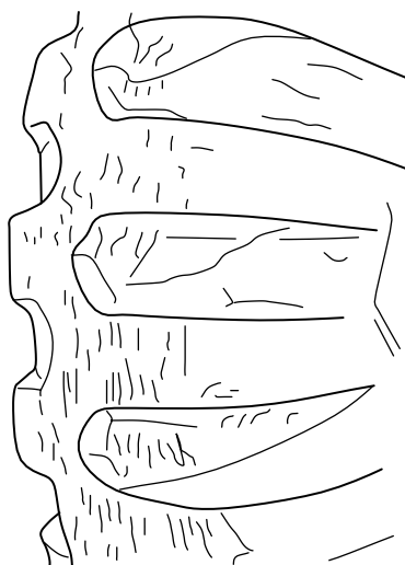
Figure 17. Oxidation of the Tire Tread
