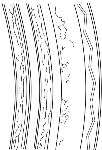
RETREAD OVER EXISTING RETREAD CONDITION
