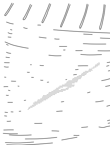
TEAR IN BEAD AREA
